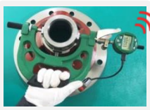
Dial snap Gage 2186-125/275 (For measuring \varnothing 105n6+0.045/+0.023/ \varnothing 270h7 0/-0.052 )
