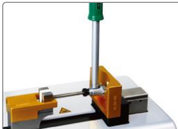
zero setting and calibration of bore gauges
