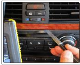
Measuring gaps on the car dashboard
