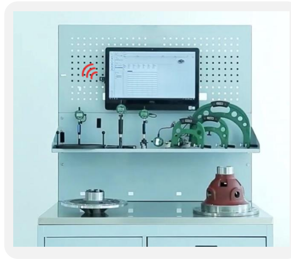
Dial snap Gage 2186-125/275 (For measuring \varnothing 105n6+0.045/+0.023/ \varnothing 270h7 0/-0.052 )
